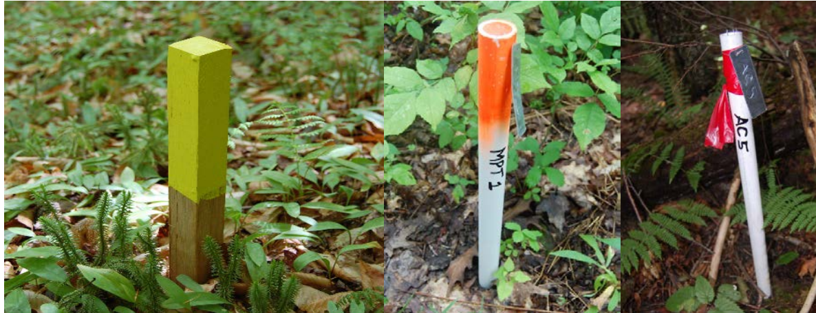
Figure 1. Mark your plot centers with pvc pipe, a wooden stake or rebar. Mark the stake using brightly colored paint, surveyors flagging or brightly colored duct tape to make it easy to relocate.
